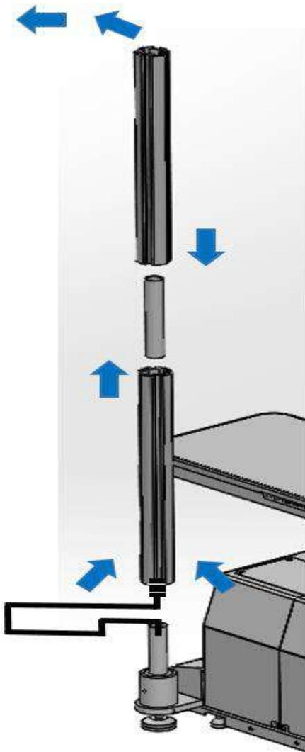
**3. Insert stand pole into the base and fix it.**
